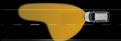
Adverse Weather Light (up to 70 km/h). Activated by wipers or a rain sensor, this setting improves vision in wet weather.
