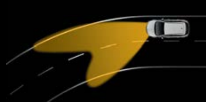
Dynamic Curve Light (any speed). The headlights turn into the curve by up to 15°. Activated by steering angle and speed.
